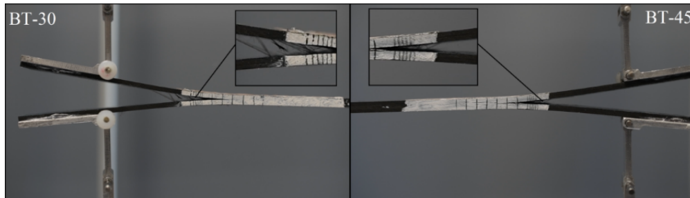
Figure 1: Experimental DCB tests conducted on elastically coupled composite laminates.
